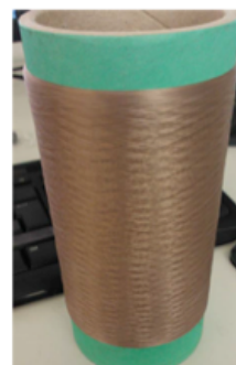
Melt spun SPEEK/PP 5:95 filaments
