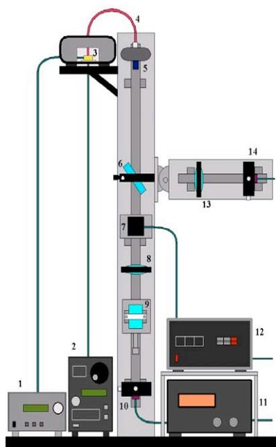
**Fig.1:** Thermal-lensing apparatus
