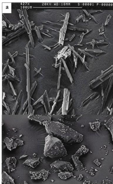
**Fig 1** SEM pictures of GV118819X as received (a) and after cooling from melt (b).
