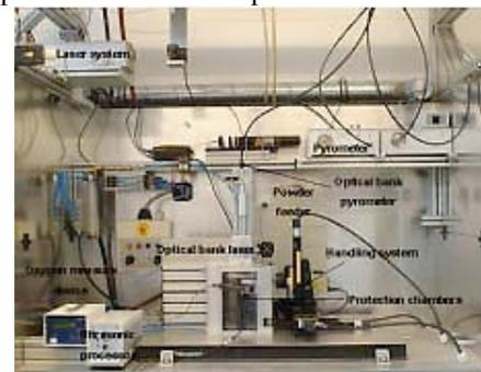
*Fig.1* Micromaking machine prototype
