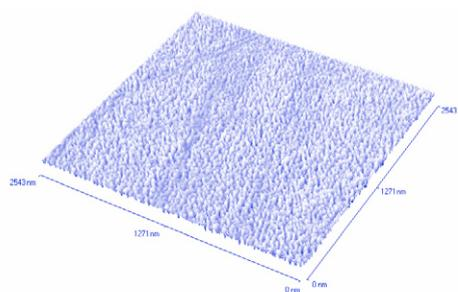
**Fig 1.** 3D AFM image of a silica wafer coated with gold nanoparticles by flame spraying of microemulsions. Mean diameter of the nanoparticles is about 35 nm.
