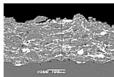
**Fig.5** Fe/Cu/WC/Co coating: SEM image
