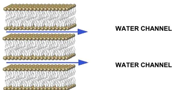
Fig. 1 Sketch of a lamellar phase
