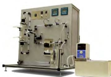
Figure 1. Bioreactor used for the synthesis of new bio-dyes
